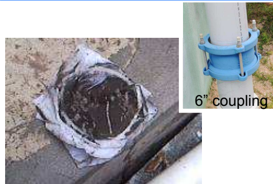
Contamination residue on the first-flush cloth filter
